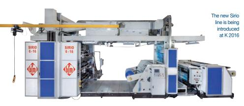
MACPLAS INTERNATIONAL AT K 2016 67 ing. The drying system includes both intercolour fans and drying tunnel, with electrical or gas heating. The nip roll section features an independent motor and chilled rollers. The winder is motorized and provided with hydraulic unloader for reels.
